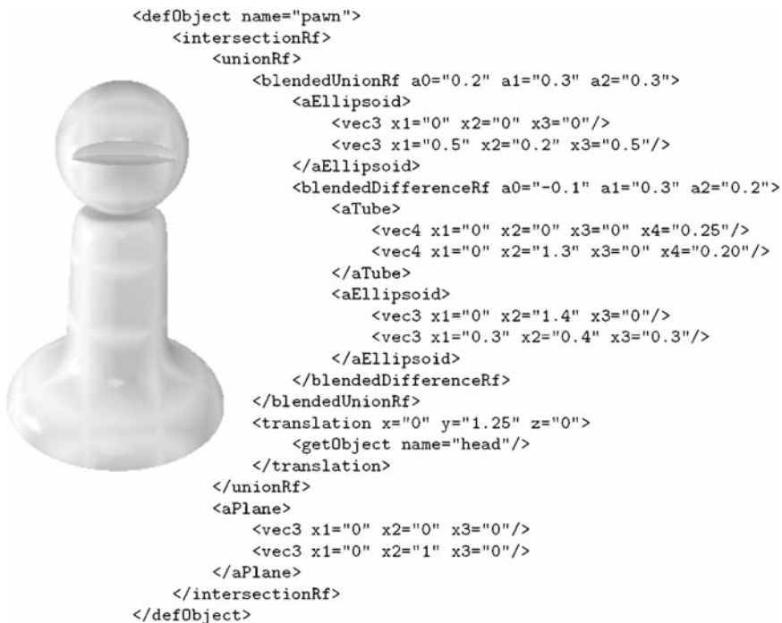
Fig. 2. Demonstration of the XISL language (script) that defines the implicit “pawn” object and its rendition.
